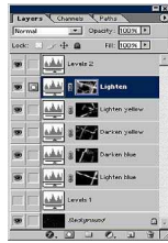
Fig. 35.— The layers palette in Photoshop for the cleaned image in Figure 34. Note that the masks for the adjustment layers have been painted in so that only the chip gaps are lightened.
