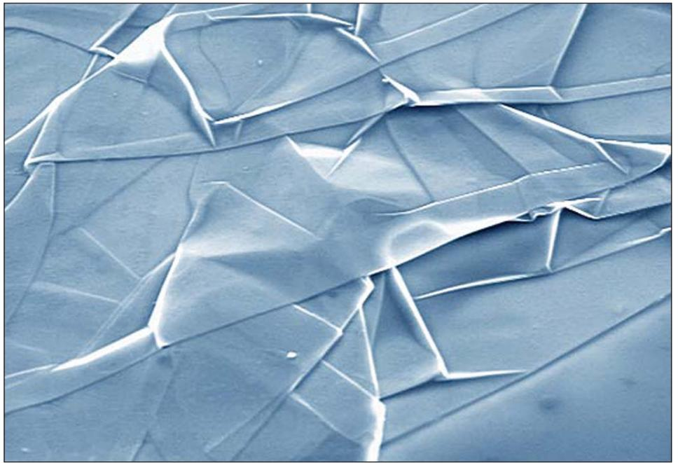
**SEM micrograph of a strongly crumpled graphene sheet on a Si wafer. It looks like silk thrown over a surface. Lateral size of the image is 20 microns. Si wafer is at the bottom-right corner. Photo courtesy K. Novoselov, University of Manchester.**
