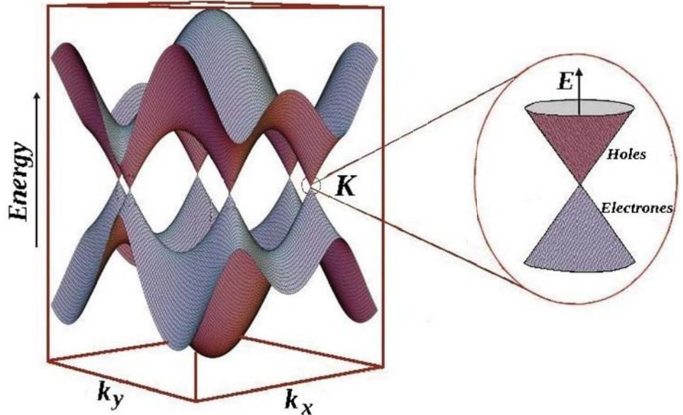
**Energy dispersion relation of graphene (as derived by Philip Wallace). The lower band is completely filled and meets the totally empty band at the K point. Illustration courtesy Tapash Chakraborty.**
