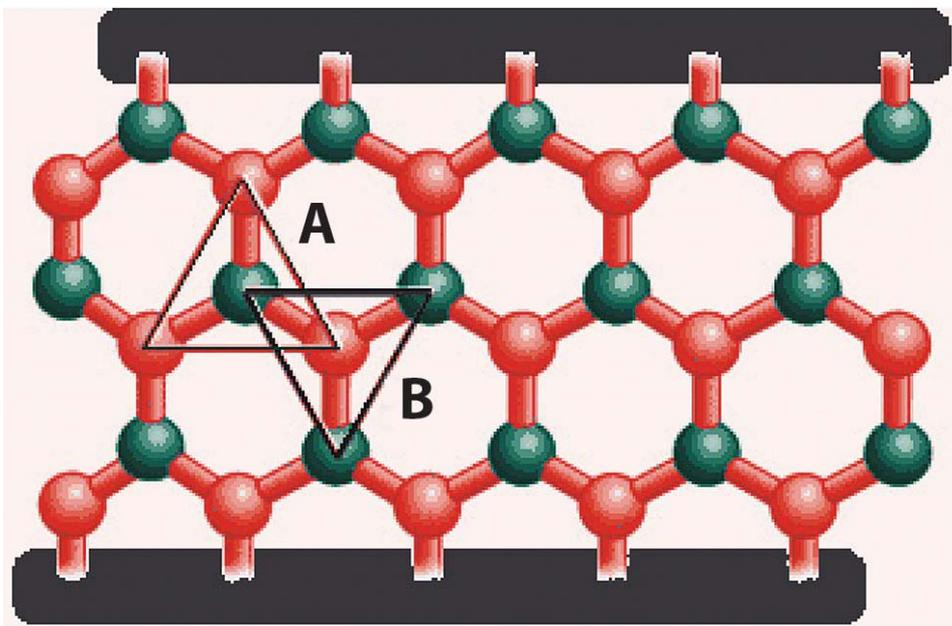
**This diagram of a graphene lattice illustrates a unit cell containing two atoms – Atom A and Atom B. Illustration courtesy Tapash Chakraborty.**
