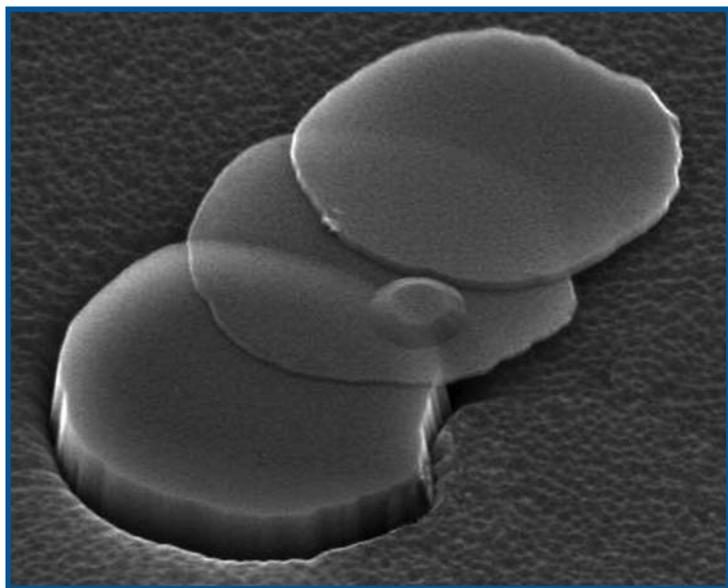
Fig. 1 Scanning electron micrograph of a fallen mesa of graphite. This is the way graphene molecules were "extracted" from bulk graphite. To be reasonably visible in SEM, a 10 nm carbon flake (30 layer thick) is shown. Courtesy of K. Novoselov, University of Manchester, <http://onnes.ph.man.ac.uk/nano/Images.html>
