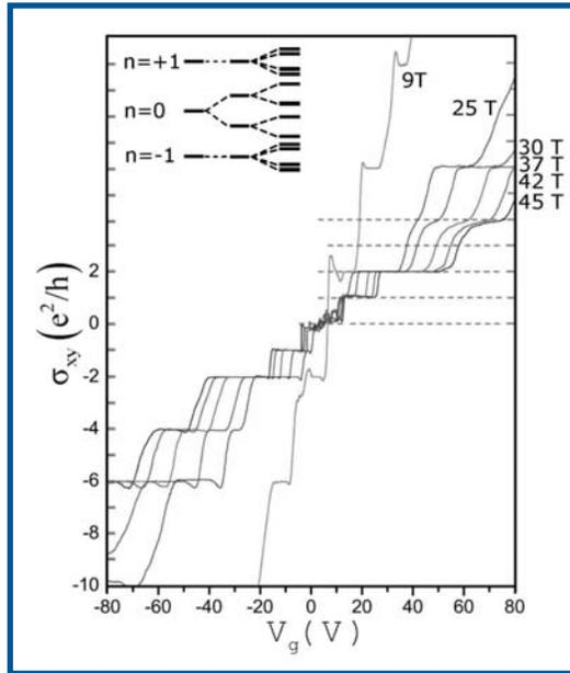
**Fig. 5** Quantum Hall effect in graphene at high magnetic fields. The plateaus at  $\nu = 0, \pm 1, \pm 4$  are resolved at these fields. Inset: Landau levels (schematic) at low (left) and high (right) magnetic fields (adapted from Ref. [9]).
