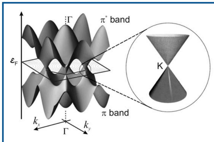
**Fig. 3** Band structure of graphene. Since we ignore the coupling between the graphene sheets, the bands depend only on  $k_x$  and  $k_y$ . The  $\pi$  band is completely filled and meets the totally empty  $\pi^*$  band at the K and K' points (Dirac points). Near these points both the bands have linear dispersion as described in the text.
