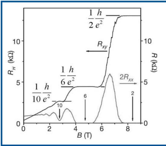
**Fig. 4** Quantum Hall effect in graphene. The Hall resistance plateaus appear at the filling factors  $\nu = 2, 6,$  and  $10$  (adapted from Ref. [8]).
