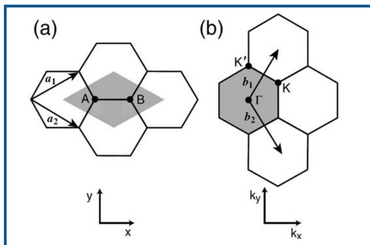
Fig. 2: (a) Graphene lattice in real space, and (b) the corresponding reciprocal lattice. The unit cell in the graphene lattice (shaded rhombus) contains two atoms A and B. The first Brillouin zone is drawn as shaded hexagon. The basis vectors of the direct lattice and the reciprocal lattice are  $a_i$  and  $b_i$  ( $i = 1,2$ ) respectively.
